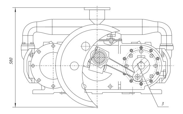
Picture 1 - Pendulum oil-free compressor KM-12-2R1. Structure.
