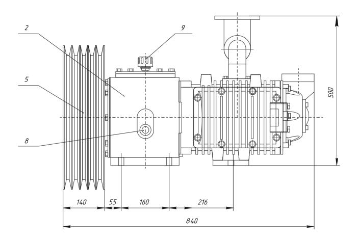
Picture 3 - Pendulum oil-free compressor KM-12-2R1. Structure.
