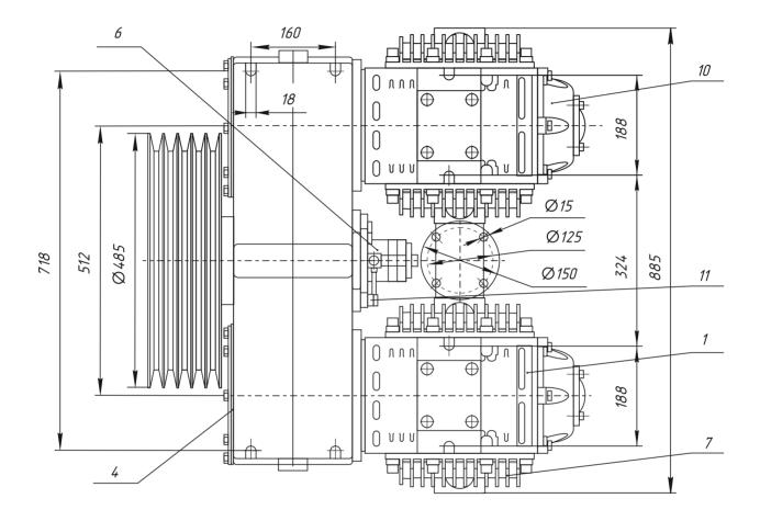
Picture 2 - Pendulum oil-free compressor KM-12-2R1. Structure.
